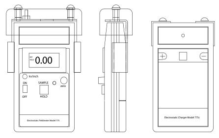
Model 775 Fieldmeter with Model 775P Plate Assembly Model 775C 1KV Charger
