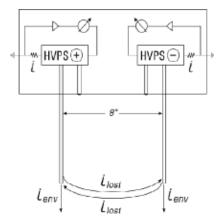
Simco-Ion design for maintaining stable ion current flow despite fluctuating environmental conditions, point erosion and point "aglomeration" (+HVPS Alarm - level set at factory).
