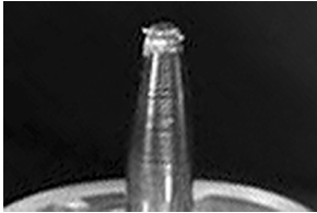
Close up of an eroded titanium emitter point
