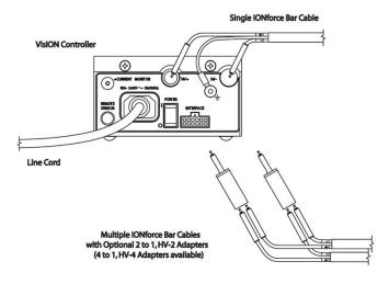
Figure 3. IONforce Bar Connections to VisION Controller Unit
