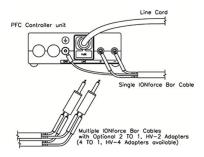
Figure 2. IONforce Bar Connections to PFC Controller Unit
