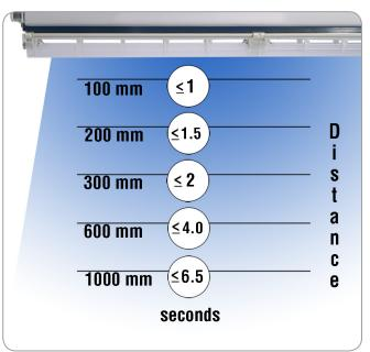
Measured using Simco-Ion CPM Model 280A w/HEPA flow (60 fpm or 0.3m/sec) & CDA flow at 50 lpm.
