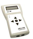
SIMCO ION MICROWIRE 5700 VERSION x.x IR MODE IR (infrared) Communications interface allows two way line-of-sight communications to the 5710 AeroBar. A 9 VDC battery (internal) is required for using the IR interface. When the HHT is turned on and not wired to the 5710 AeroBar it will automatically switch to IR mode. The IR range is approximately 8 feet.
