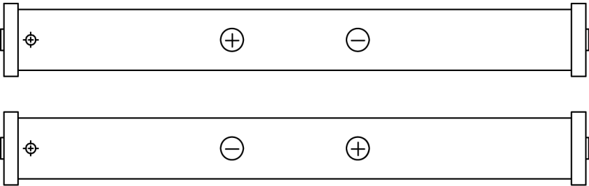
Figure 3. Recommended Installation for 11 inch AeroBar
